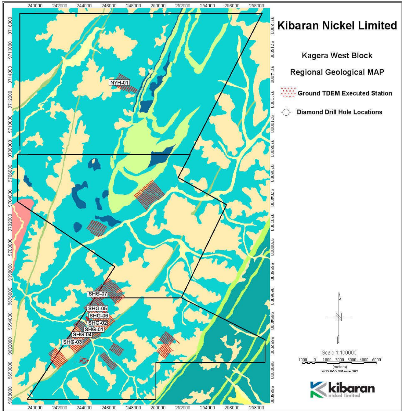
Figure 4: TDEM over Regional Geological Map. The red polygons indicate areas covered by the TDEM survey. Only limited coverage of the large claim was completed in the initial program.
